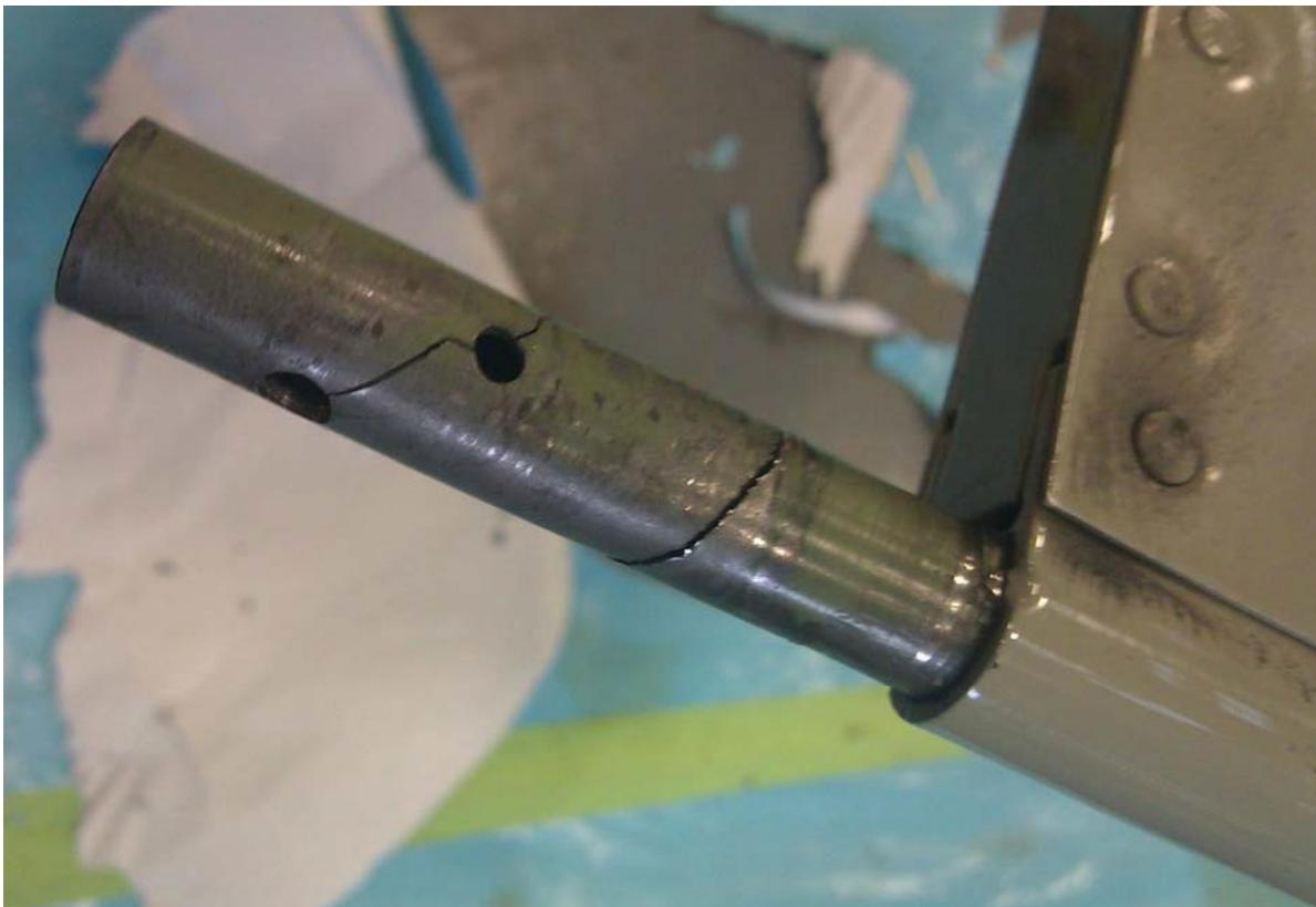
Cessna 208B, Cracked Inertial Vane Shaft, ATA 7160
